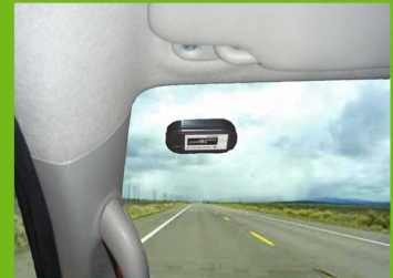
Typical window fitment of iTrakII-TX
